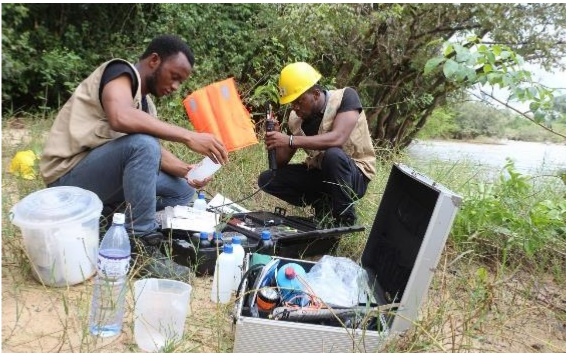
Figure 4-14: INTEGEMS staff calibrating the HI 9829 Multi-parameter Meter along the Sewa River
